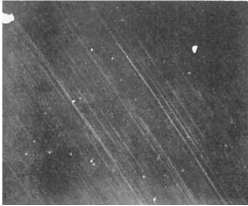
Fig. 2. The microphotograph of friction surface of stainless steel rubbed against pure PTFE for 1 h (100 \times ).
