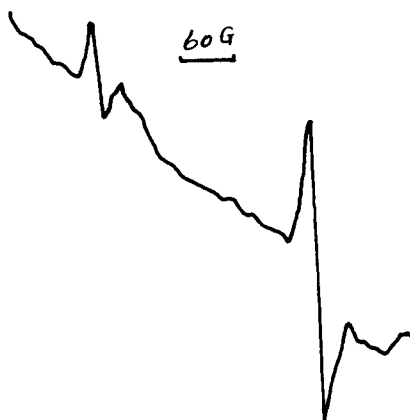
Fig. 11. The ESR spectrum of JS material wear debris collected from stainless steel/JS material rubbing for 2 h.
