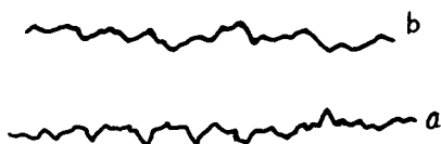
Fig. 9. ESR spectra of fragments and wear debris of pure PTFE: (a) PTFE fragments cut with a shive; (b) PTFE wear debris collected from pure PTFE rubbing against stainless steel for 1 h.
